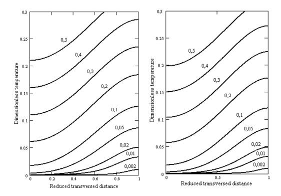
**Fig. 1**. Dimensionless temperature profiles for adiabatic walls, *n*=1 (Newtonian fluid), *NBr*=1
